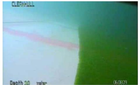
Partly cleaned hull with algae fouled area
